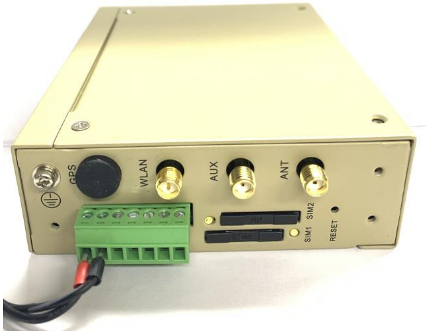
Figure 3-5 Installing the Power Supply
